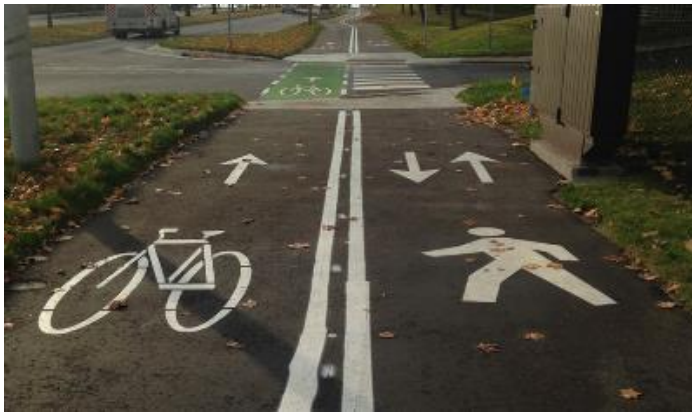
Figure 18. Integration of pedestrian and bicycle lanes
